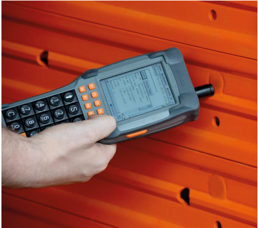
The reading device reading out data from the panel
