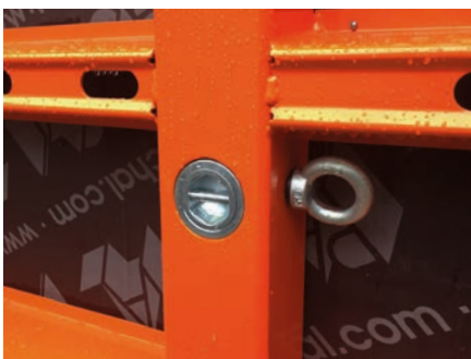
Clamping unit flush mounted in the panel frame
