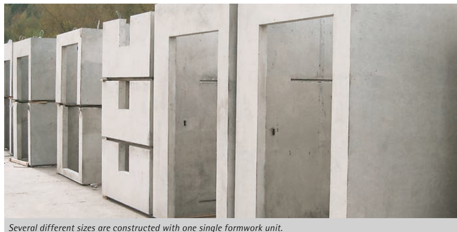
Several different sizes are constructed with one single formwork unit.
