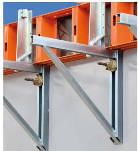
Fixing to the wall is achieved either by using wall-plugs with bolts or with DW 15 tie rods.
