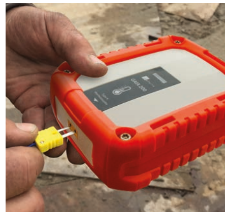
The sensor cable is attached directly to the reinforcement and connected to the radio transmitter.
