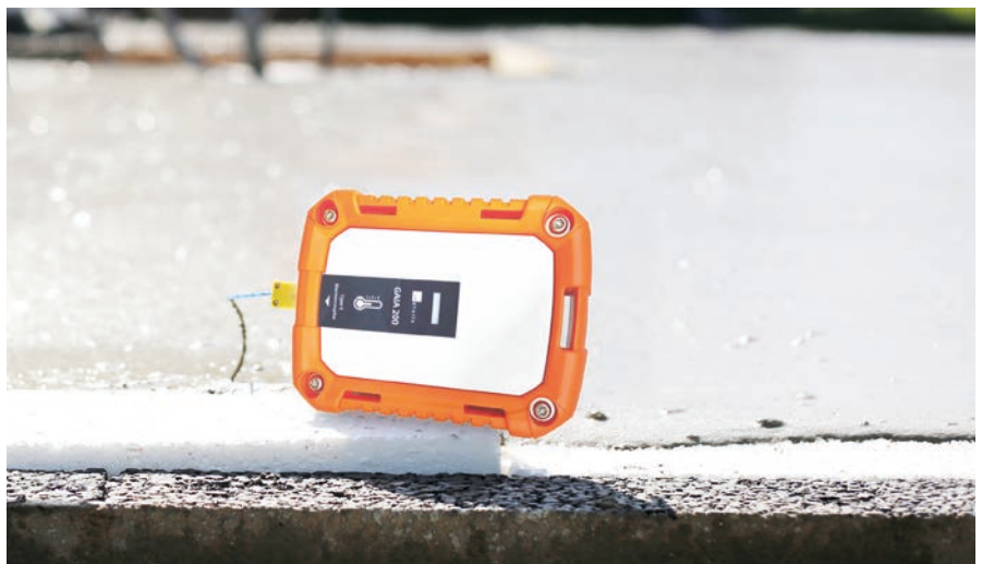
The sensor sends the measurement data via the Sigfox network using wireless technology.
