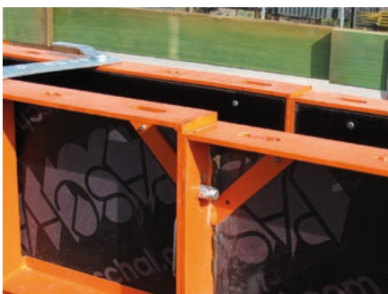
The integrated oblong holes in the element frame allow a height offset of up to 2 cm for uneven installation surfaces.
