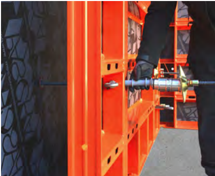
For single-sided anchoring, the tie rod together with the tube, the guide bushing and plate with ball-and-socket joint are turned into the clamping unit of the outer formwork.
